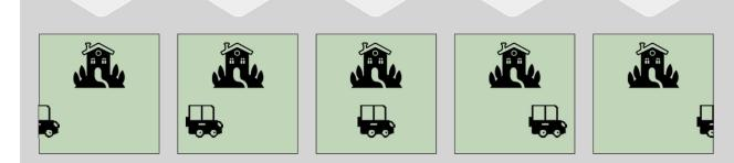
UAI transforms data into world coordinates so that static objects stay at a fixed position and dynamic objects move less. Labeling gets much, much easier this way!
