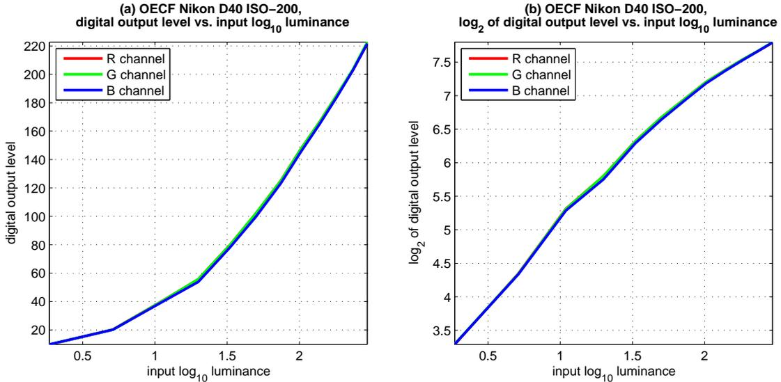
Figure 3: (a) OECF - Nikon D40, ISO 200, digital output level vs. input  $\log_{10}$  luminance, (b) OECF - Nikon D40, ISO 200,  $\log_2$  of digital output level vs. input  $\log_{10}$  luminance
