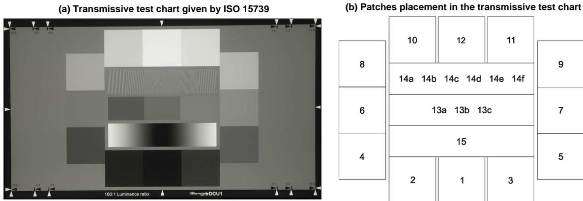
Figure 2: Noise and OECF measurement test chart and patches placement, (a) Transmissive test chart given by ISO 15739, (b) Patches placement in the transmissive test chart given by ISO 15739
