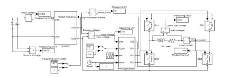
Fig.4 Simulation analysis diagram of matrix converter
