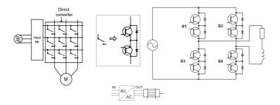
Fig. 1 Block diagram of the matrix converter
