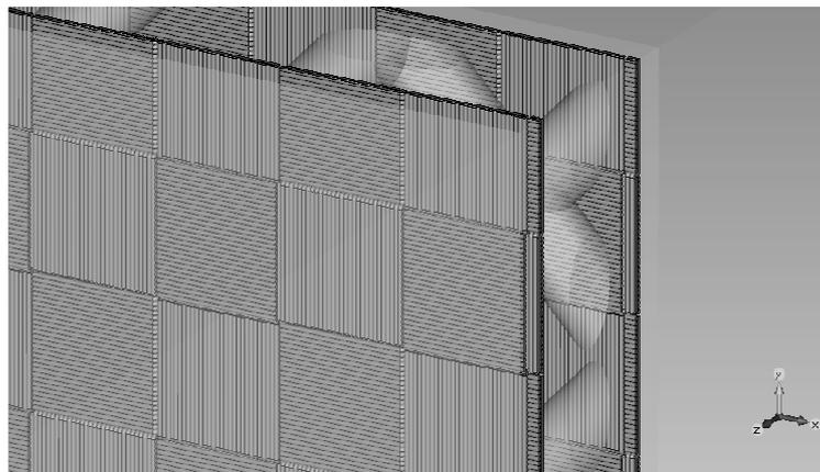
Figure 5: Detailed three dimensional model of composite material with carbon fiber reinforcement. Simulated in CST Microwave Studio.
