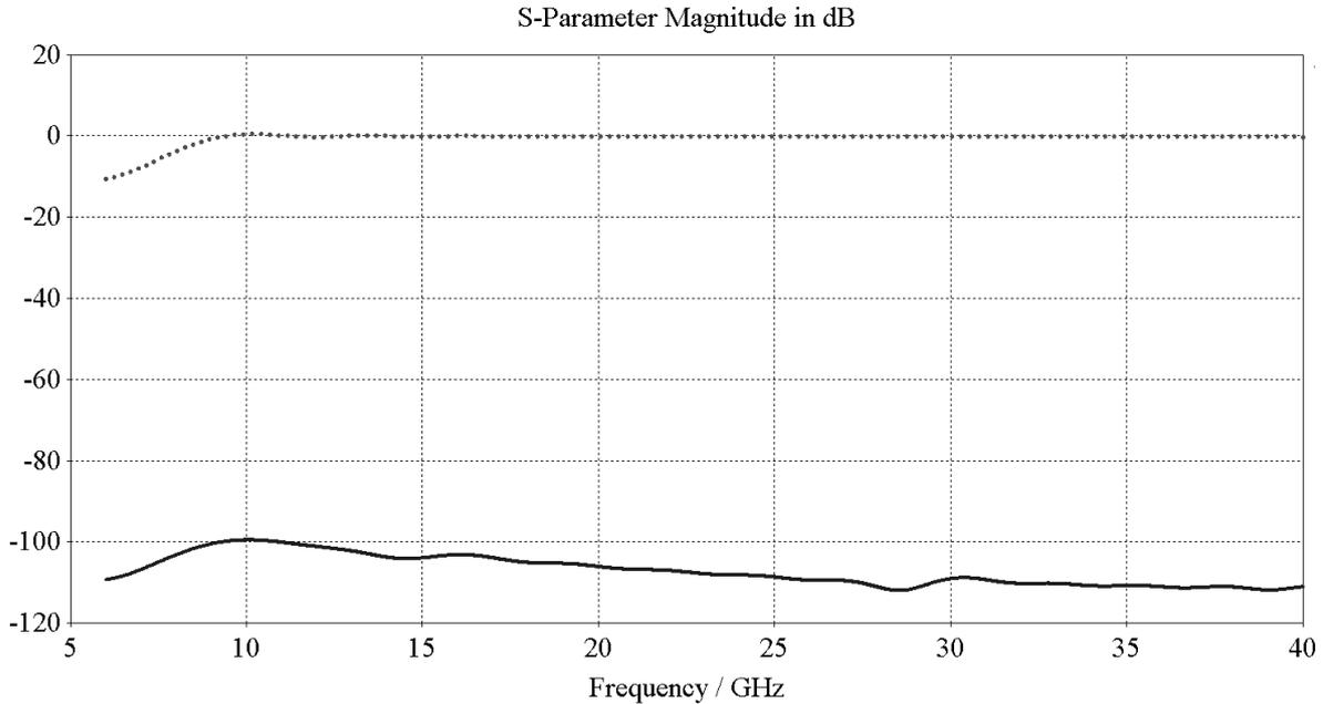
Figure 6: Transmission coefficients of 3D model of composite material with carbon fiber reinforcement. Dotted line is reflection coefficient, solid line is transmission coefficient. Simulated in CST Microwave Studio.
