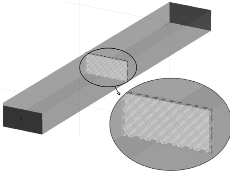
Figure 1: Simple three dimensional model of composite layer. Simulated in CST Microwave Studio.
