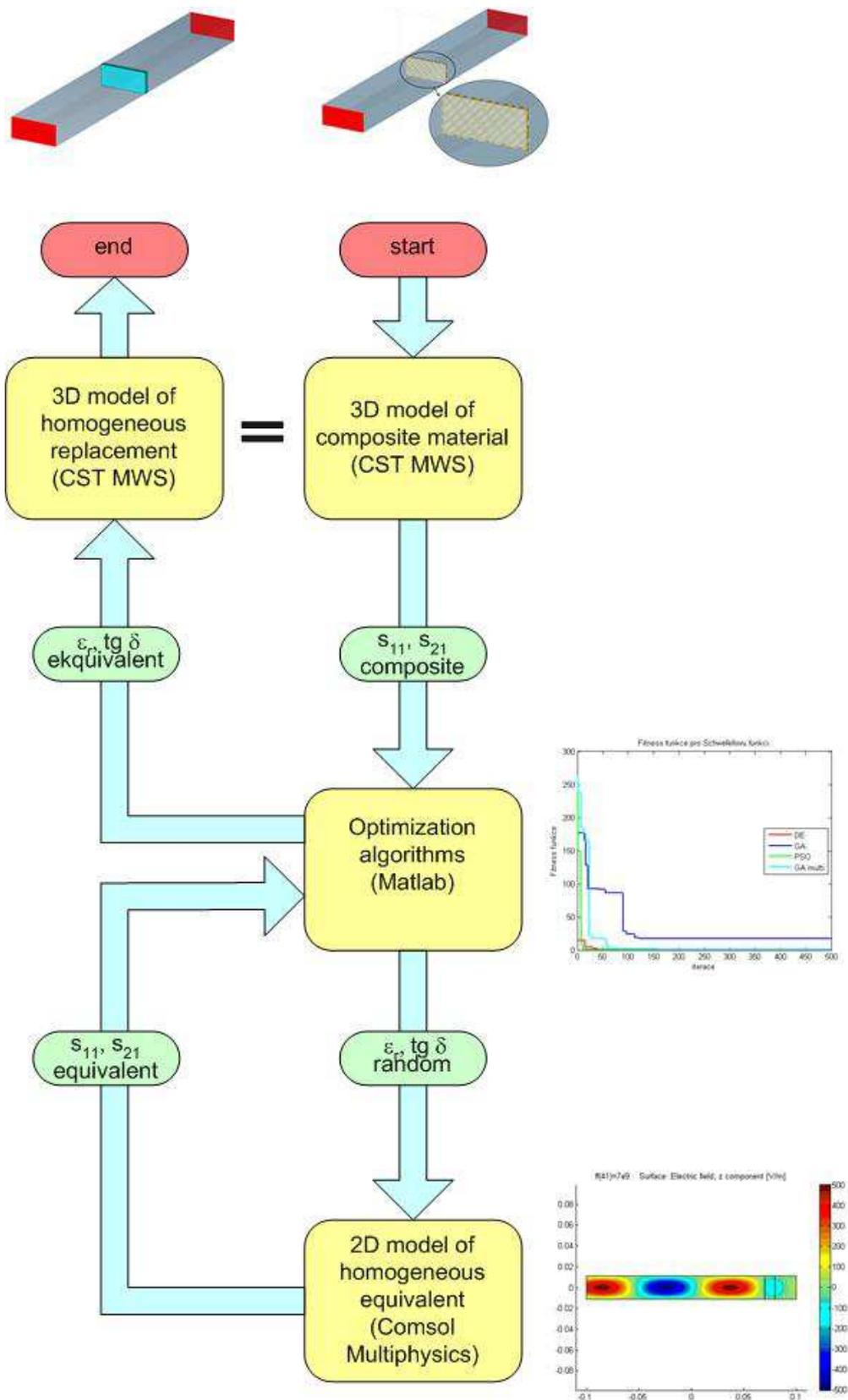
Figure 7: Flow chart of the synthesis of the homogeneous equivalent of the composite material.
