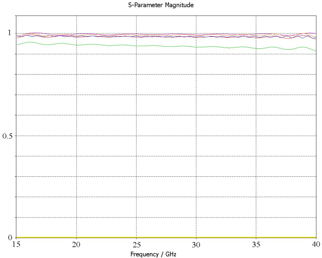
Figure 8: Reflection coefficients of replacements achieved by different optimization methods in comparison with originally reflection coefficients of composite material (blue line). (GA - orange, NPGA - violet, DE - red, PSO - green). Transmission coefficients are yellow. Simulated in CST Microwave Studio.
