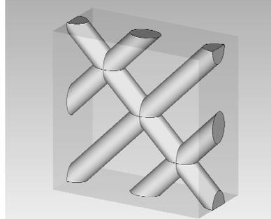
Figure 4: Elementary cell of the simple three dimensional model of the composite material. Simulated in CST Microwave Studio.
