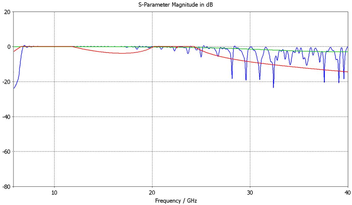
Figure 2: Reflection coefficient of the simple model of the composite material. Red line: frequency solver, green line: frequency domain with periodic boundary conditions, blue line: time domain solver. Simulated in CST Microwave Studio.
