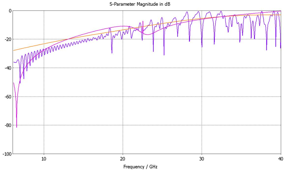
Figure 3: Transmission coefficient of simple model of composite material. Violet line: frequency solver, orange line: frequency domain with periodic boundary conditions, blue line: time domain solver. Simulated in CST Microwave Studio.
