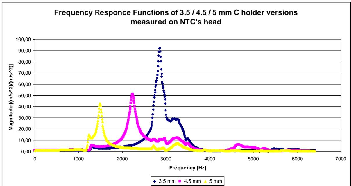
Figure 10: Resonant frequency is falling down when part is longer
