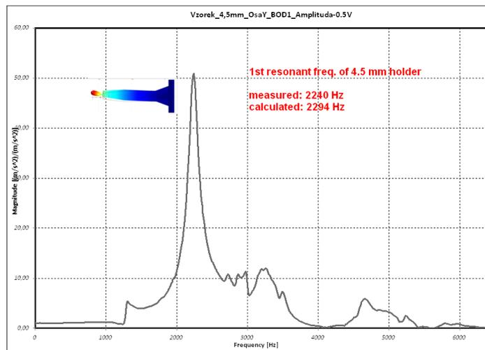
Figure 9: Example of FRF measured on the NTC's head
