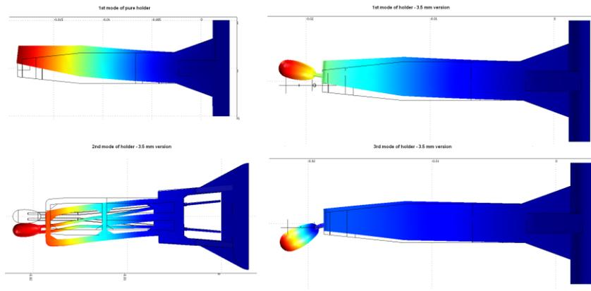
Figure 6: Vibration modes of C concept holder
