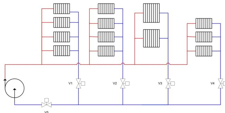
Figure 1: Configuration of the hydronic system for the experiment
