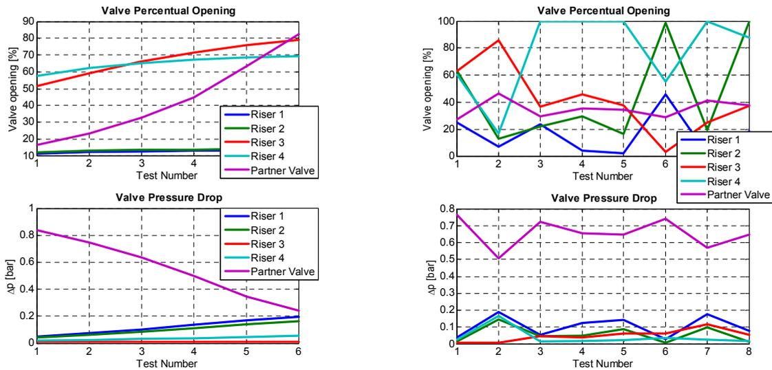
Figure 3: Achieved results – valve openings and differential pressures (for the same targets on the left picture, for random targets on the right picture)
