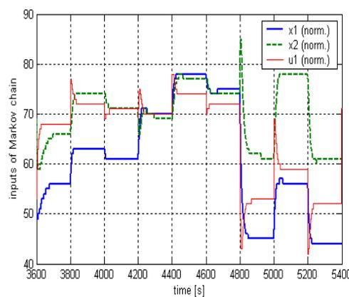
Figure 4: Discretized and normalized system variables during the diagnosis
