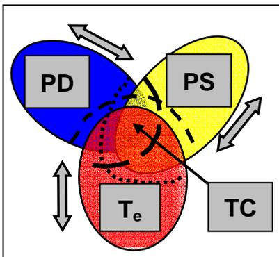
Figure 1: Control objective – *TC* area. Thermal comfort area (indicated in cross-section as *TC*) represents desired states of turbulence intensity (*PD*-index) and desired local air velocity (*PS*-index) chosen under given indoor thermal environment  $T_e$  – effective temperature). In joint areas are indicated also respective error bands (dashed lines).
