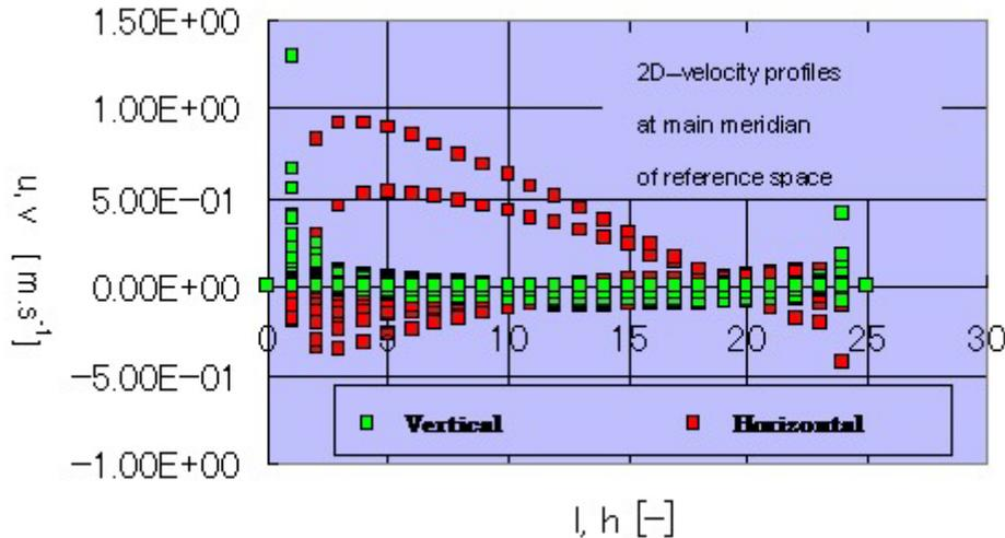
Figure 2: Indoor air velocity profiles in investigated space's main meridian cross-cut induced by thermal buoyancy. 2D-velocity field of air movement;  $ACH = 2.0$ .
