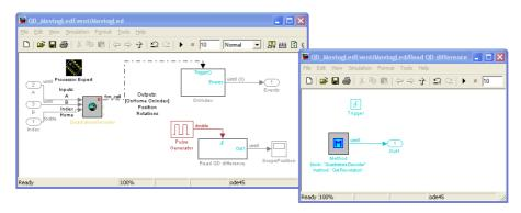
Figure 6: Submodel with QD block and an external QD method in different time domain
