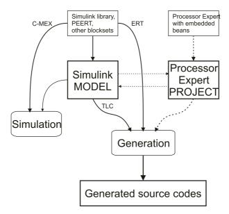
Figure 1: The SESA flow for generation code from a Simulink model
