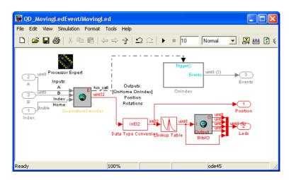
Figure 5: Model with a Quadrature Decoder periphery with interrupts
