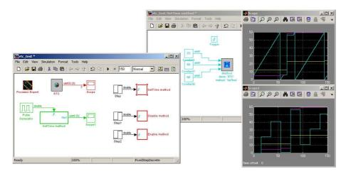
Figure 7: Model with RTC block and several external methods
