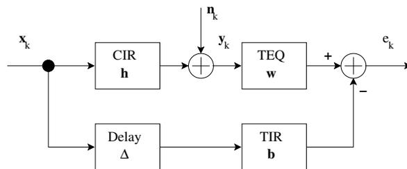
Figure 1: System model of TEQ with MSE optimization
