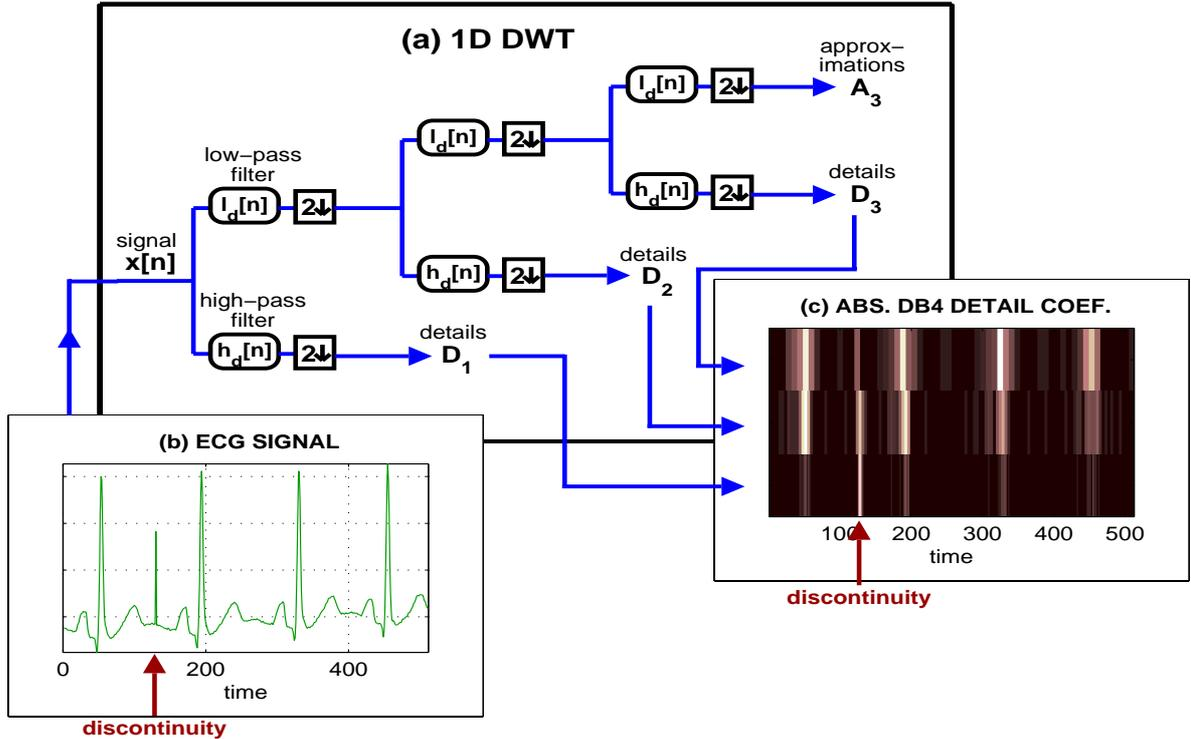
Figure 1: Discontinuity detection in the ECG signal applying wavelet analysis and presenting (a) one-dimensional wavelet subband coding scheme, (b) ECG signal with a discontinuity, and (c) absolute detail decomposition coefficients using the *db4* wavelet function
