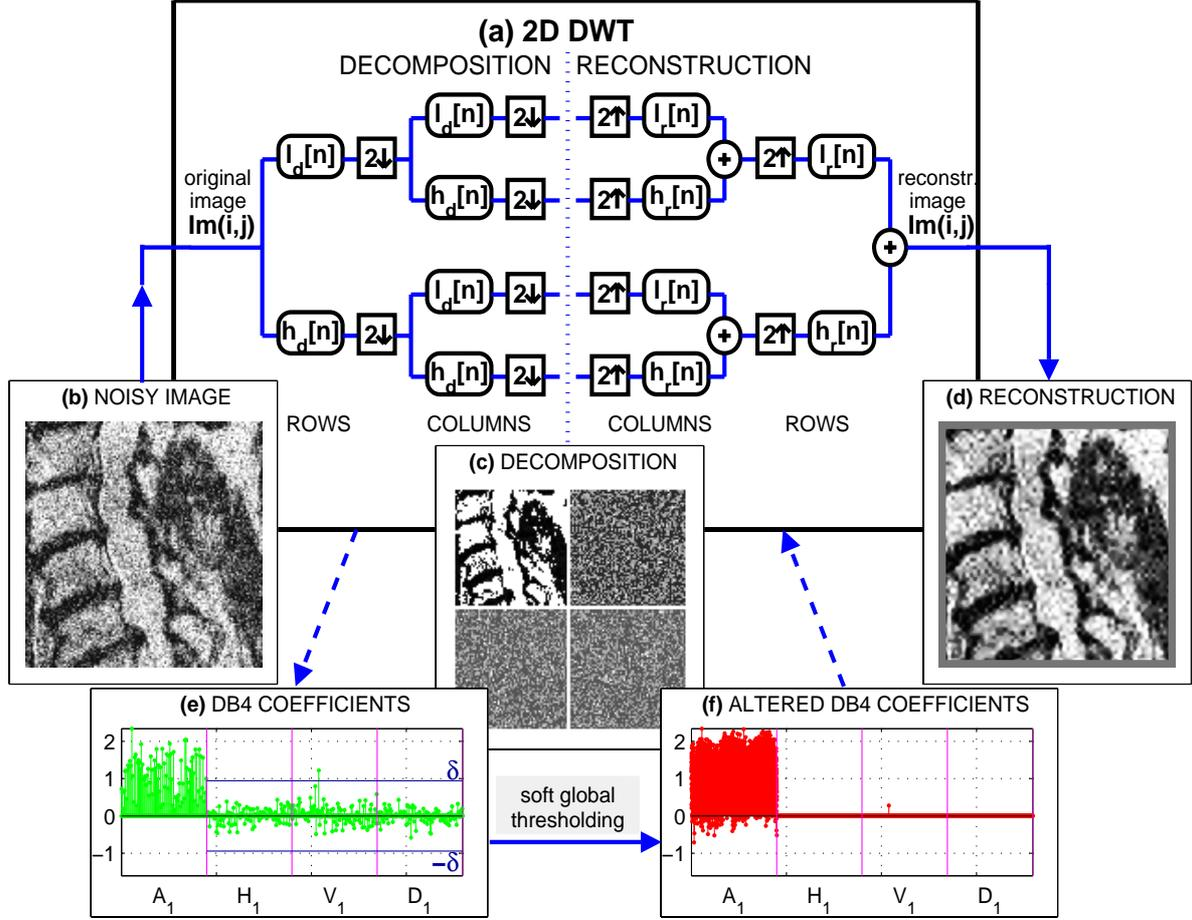
Figure 3: MR image enhancement by thresholding of the wavelet decomposition coefficients presenting (a) one-dimensional wavelet subband coding scheme, (b) noisy MR image, (c) first level decomposition using the *db4* wavelet function, (d) reconstructed and interpolated image, (e) absolute *db4* decomposition coefficients, and (f) thresholded decomposition coefficients used for image reconstruction
