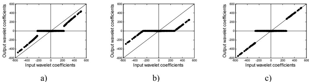
Figure 3: Transfer function, band HL3, a) MAP estimator, b) soft thresholding, c) hard thresholding
