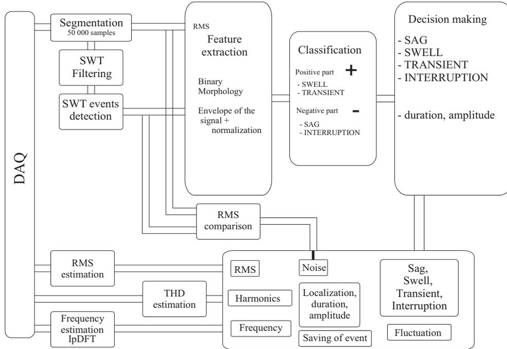
Figure 1: PQ monitoring system block diagram
