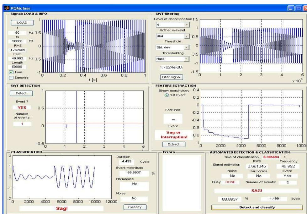
Figure 4: GUI window for detection and classification of PQ disturbances
