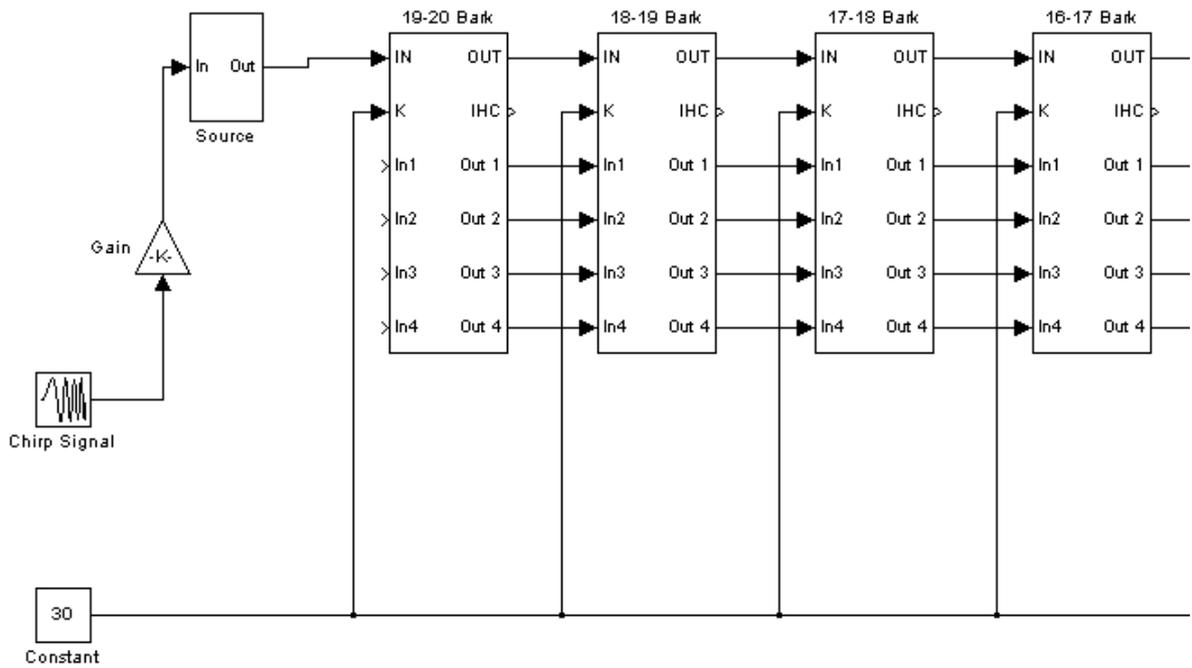
Figure 4: Top level of the cochlear model, the input plus four critical band blocks.
