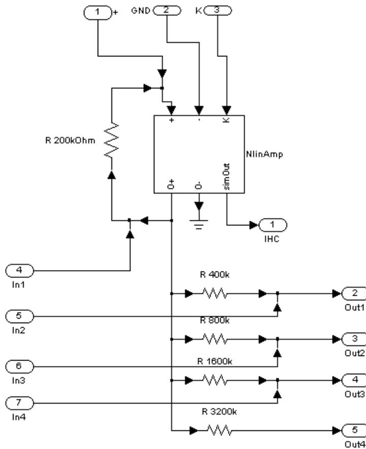
Figure 9: A single OHC circuit, detailed view.
