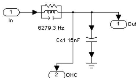
Figure 6: A single resonator included in the BM circuit.
