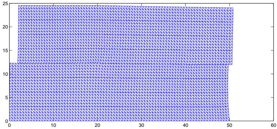
Figure 3: The deformations (enlarge factor is 50)
