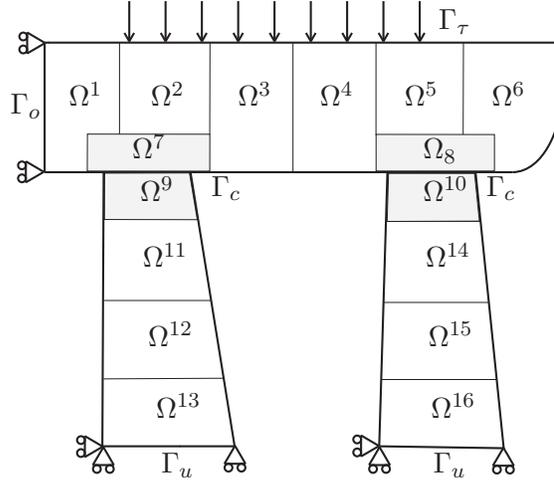
Figure 1: The contact problem with decomposition
