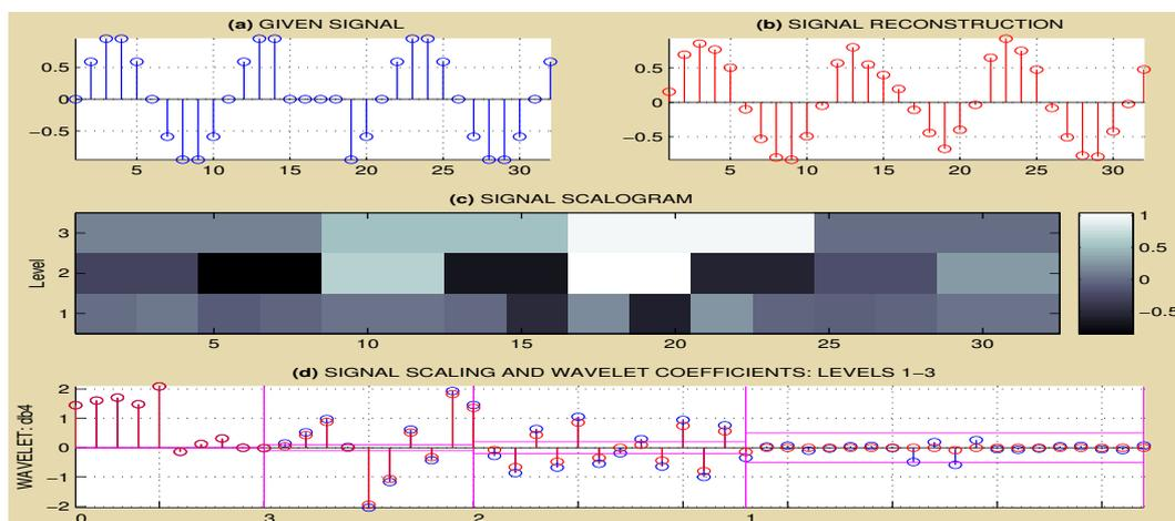
Figure 3: Simulated signal de-noising presenting (a) given signal, (b) reconstructed signal, (c) signal decomposition into two levels, and (d) wavelet coefficients thresholding
