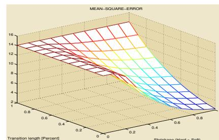
Figure 5: The study of the effect of different transition period and shrinkage level and their optimization to minimize the error between the original and de-noised signal
