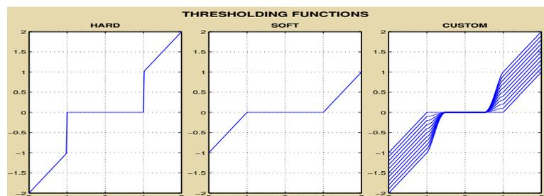
Figure 4: Hard and soft thresholding functions in comparison with custom functions allowing the selection of the transition period and shrinkage level and their optimization to minimize the error between the original and de-noised signal
