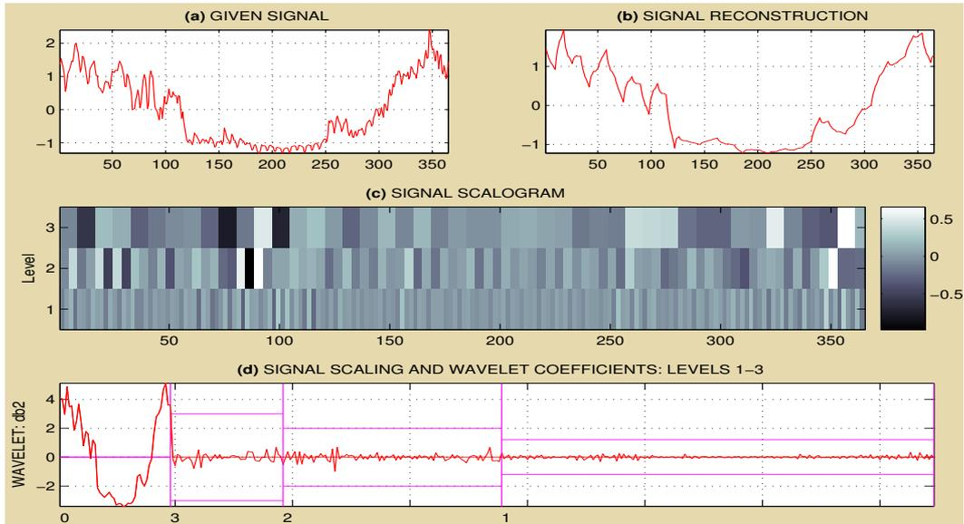
Figure 9: Principle of a gas consumption signal decomposition, thresholding and reconstruction
