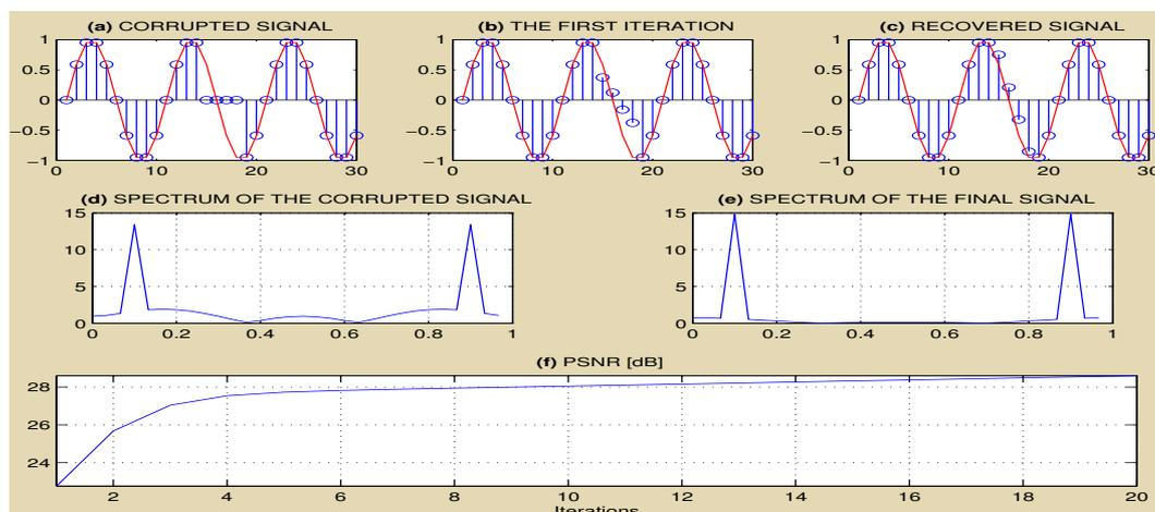
Figure 6: Simulated signal recovery process presenting (a) corrupted signal, recovered signal after (b) the first and (c) the final iteration of the recovery algorithm, spectrum estimation of the (d) initial and (e) the final signal (after 20 iterations), and (f) the peak-signal-to-noise-ratio evolution
