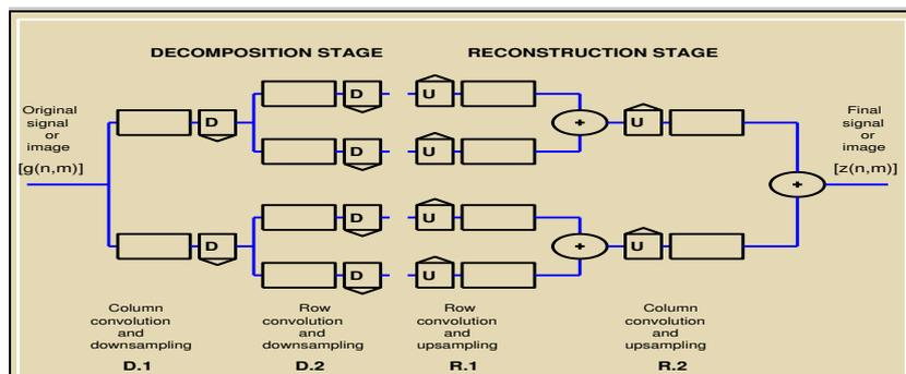
Figure 2: The principle of signal or image decomposition and reconstruction by wavelet transform
