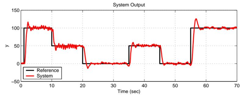
Figure 10: Reference tracking and model probability estimation - Classical LQ
