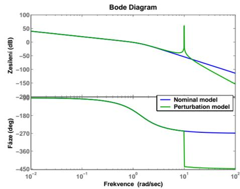
Figure 9: Bode diagrams - nominal and perturbation model
