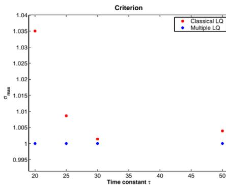
Figure 4: Maximum singular values of close loop
