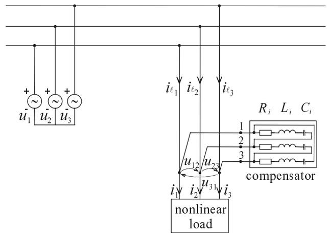
Fig. 1. Three-phase circuit structure.
