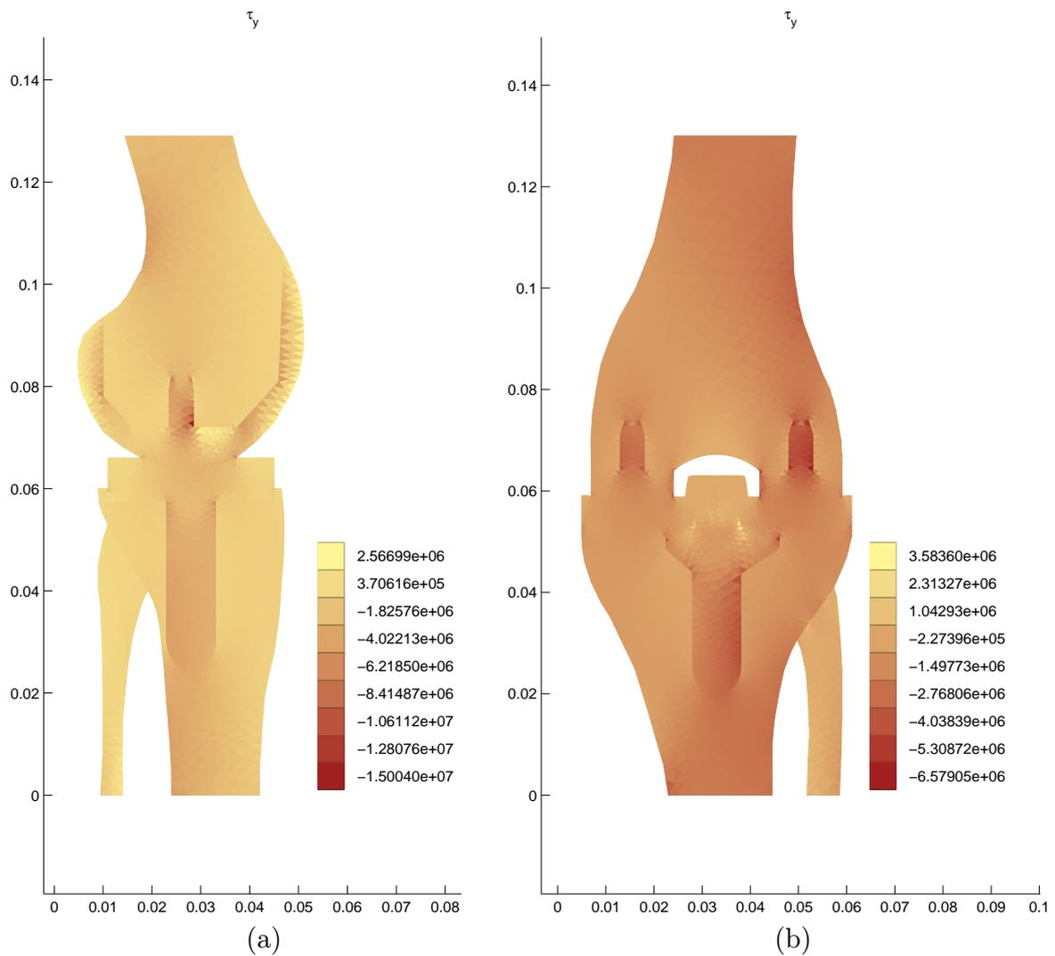
**Fig. 3.** The vertical stress tensor components, (a) the sagittal cross-section, (b) the frontal cross-section
