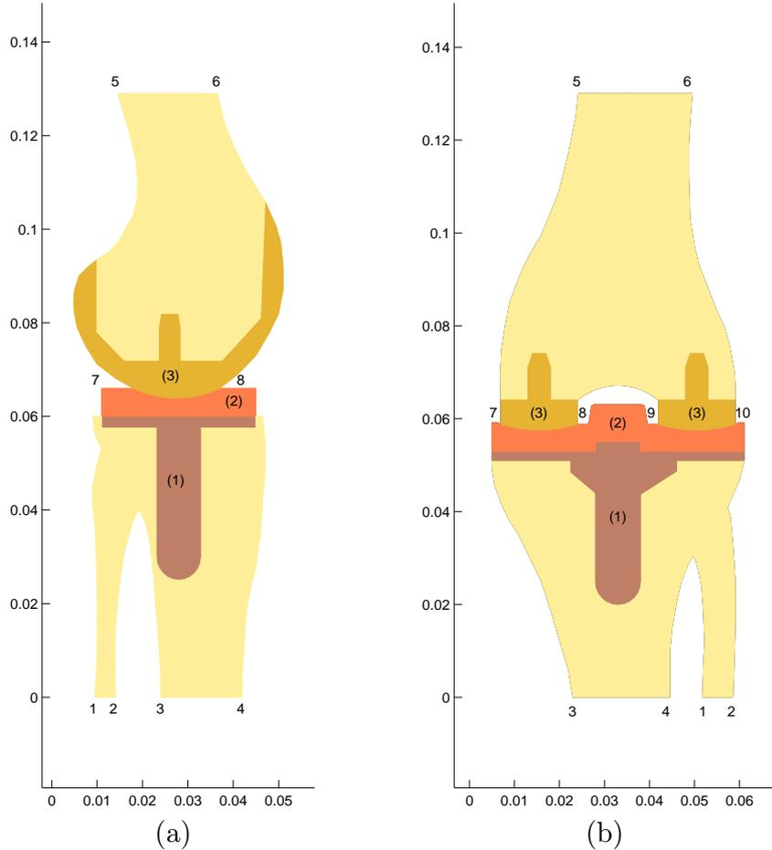
**Fig. 1.** The model of the artificial knee replacement, (a) the sagittal cross-section, (b) the frontal cross-section
