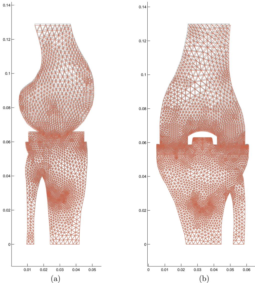
**Fig. 2.** The deformations (enlarging factor is 10), (a) the sagittal cross-section, (b) the frontal cross-section
