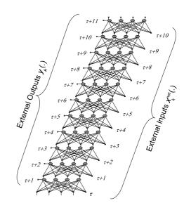
Figure 4: In time unfolded recurrent network with 11 time layers
