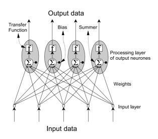
Figure 1: Architecture of linear network and structure of the neuron
