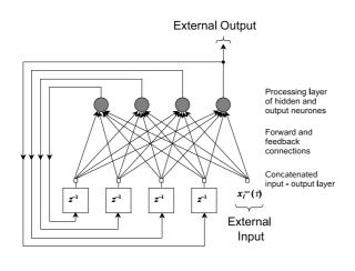
Figure 3: Architecture of recurrent network with one external input and one output [4]
