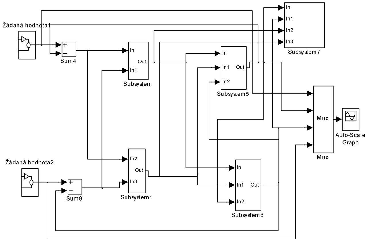
Fig 3 Simulation diagram for adaptive control of the two input – two output system
