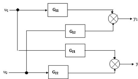
Fig. 1 Double input double output system – “P” structure
