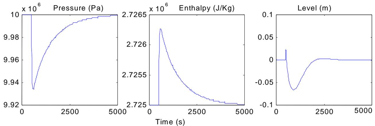
Responses in drum boiler for step increase of 5 kg/s in steam flow
