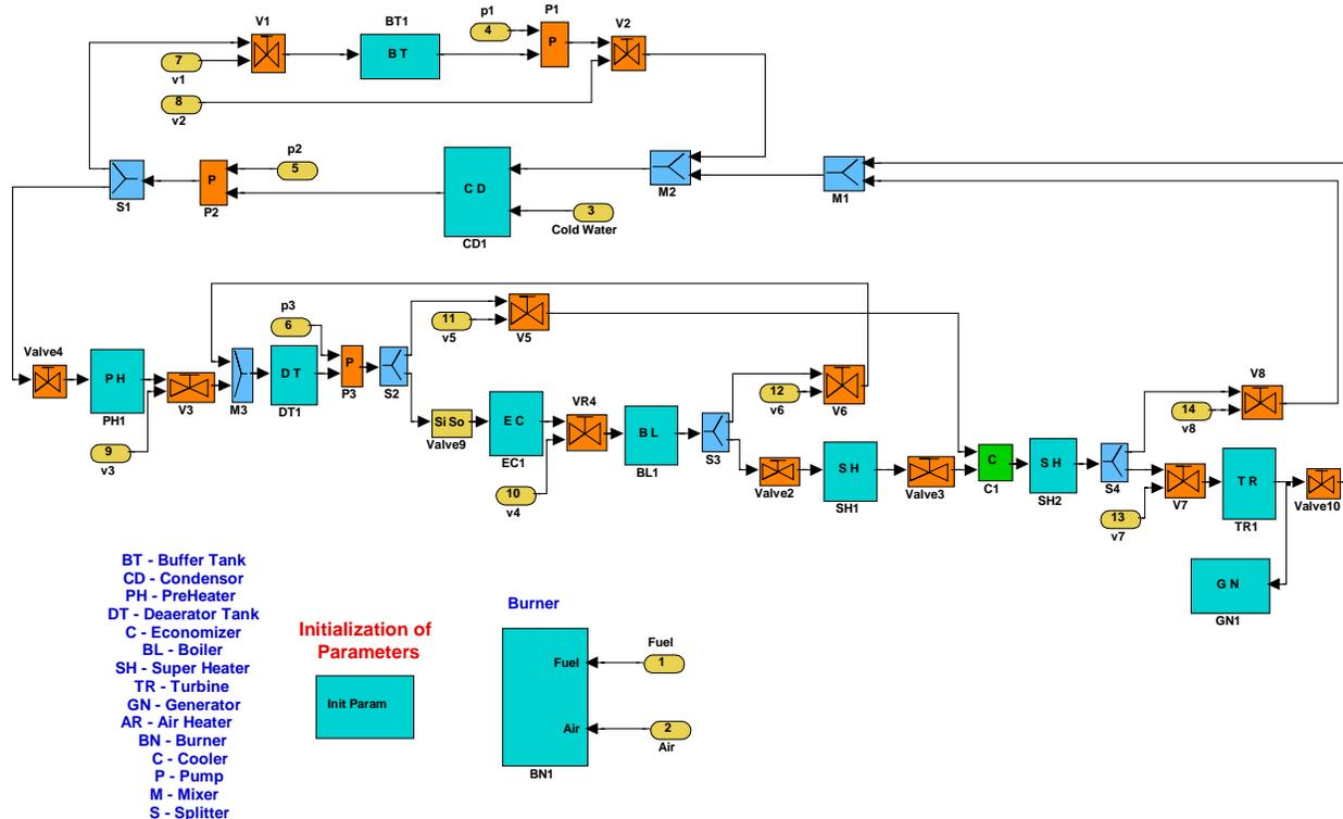
Fig. 4 Matlab/Simulink diagram of a Thermal Power Plant
