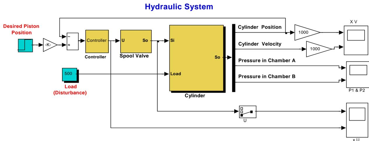
Fig. 6 Matlab/Simulink diagram of a differential hydraulic actuator
