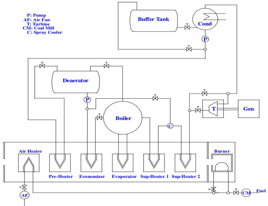
Fig. 3 Functional scheme of a Thermal Power Plant
