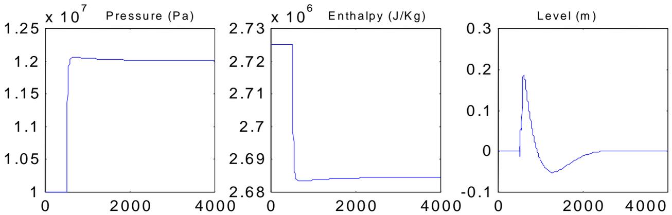
Responses in drum boiler for step increase of desired pressure
