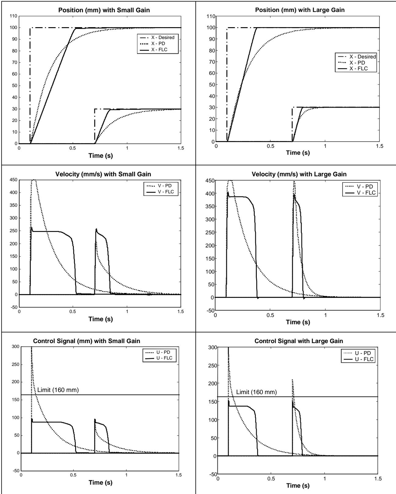
Fig. 8 Comparison of PD and FL control for different gains, step sizes and velocity limitations
