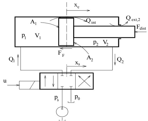
Fig. 5 Schematic diagram of a differential hydraulic cylinder
