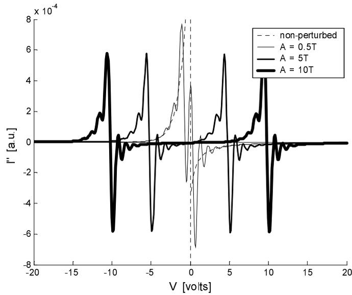
Fig.2 Second derivatives of the probe characteristic distorted by rectangular oscillations of the probe potential.
