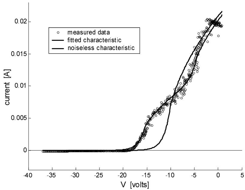
Fig.3 Measured and computed probe characteristics with the probe potential modified by rectangular oscillations.
