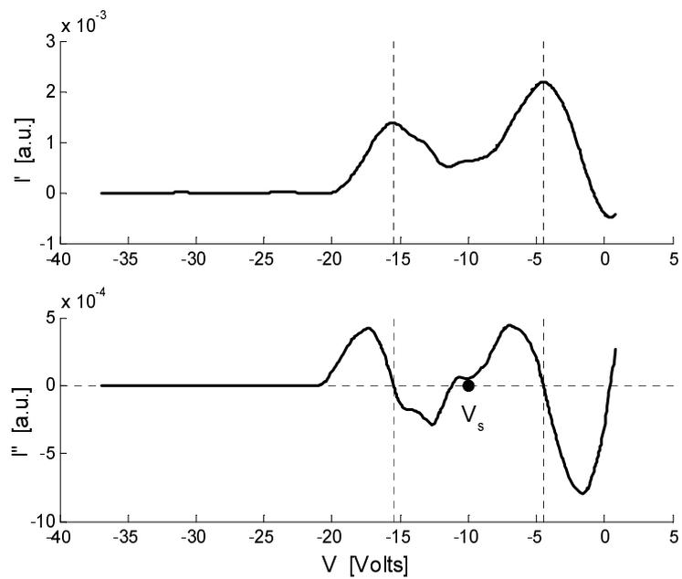
Fig.4 First and second derivatives of measured probe characteristic distorted by rectangular oscillations of the probe potential.
