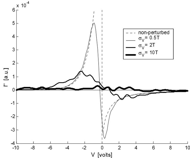
Fig.1 Second derivatives of the probe characteristic distorted by Gaussian fluctuation of the probe potential.
