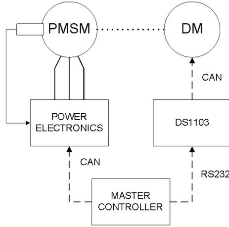
Figure 2: Hardware Structure of Laboratory Stand
