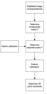
Figure 1: The general flowchart of designed system for reconstruction 3D model.
