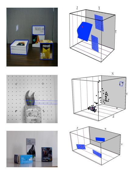
Figure 5: In first column are images of the scene. In second column are resulting reconstruction. Red marks represent location of selected point in space.
