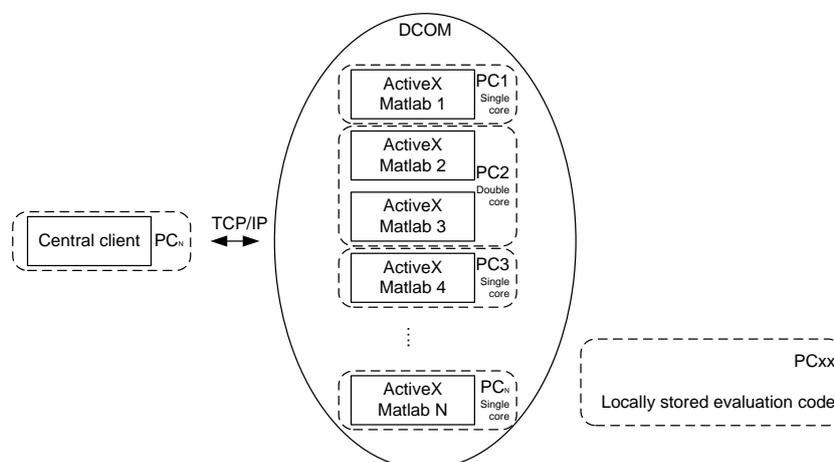
Figure 1: Client server structure of DCOM model of ActiveX Matlab objects
