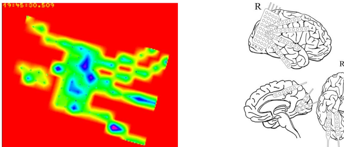
Figure 4: Example of brain mapping using signal changes detectors. Screenshot of BACD visualization on left and physical placement of visualized signal electrodes at the brain on right.
