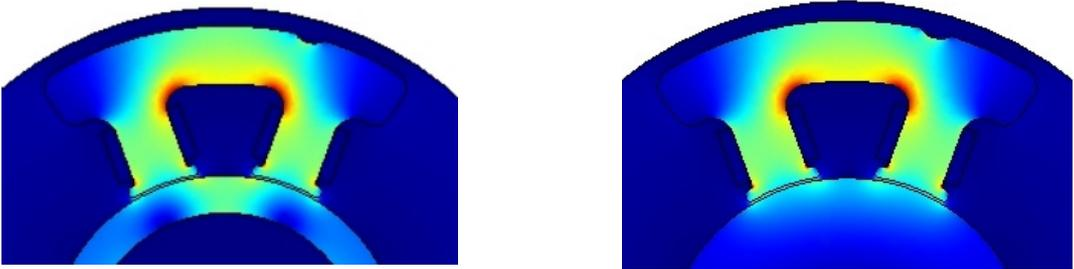
Figure 3: Magnetic flux density in the selected stator with two types of the rotor
