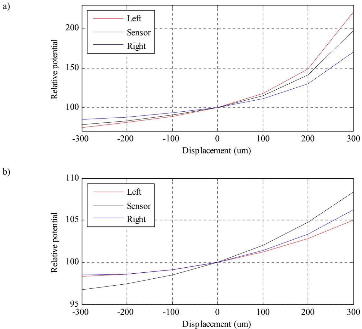
Figure 6: Relative magnetic field potential vs. rotor displacement
