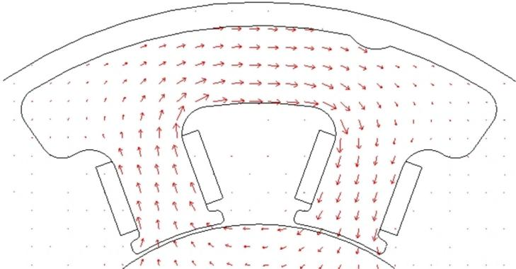
Figure 2: Magnetic flux density in the selected stator
